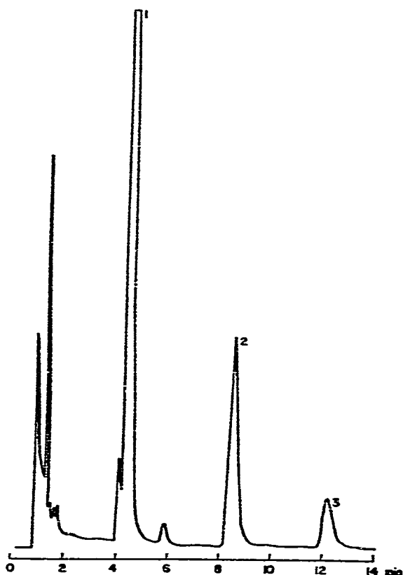
Fig. 1. Gas chromatogram of rainbow trout exposed to 15 ppm aminocarb for 144 h. Peaks: 1 = aminocarb; 2 = AM; 3 = MA.
